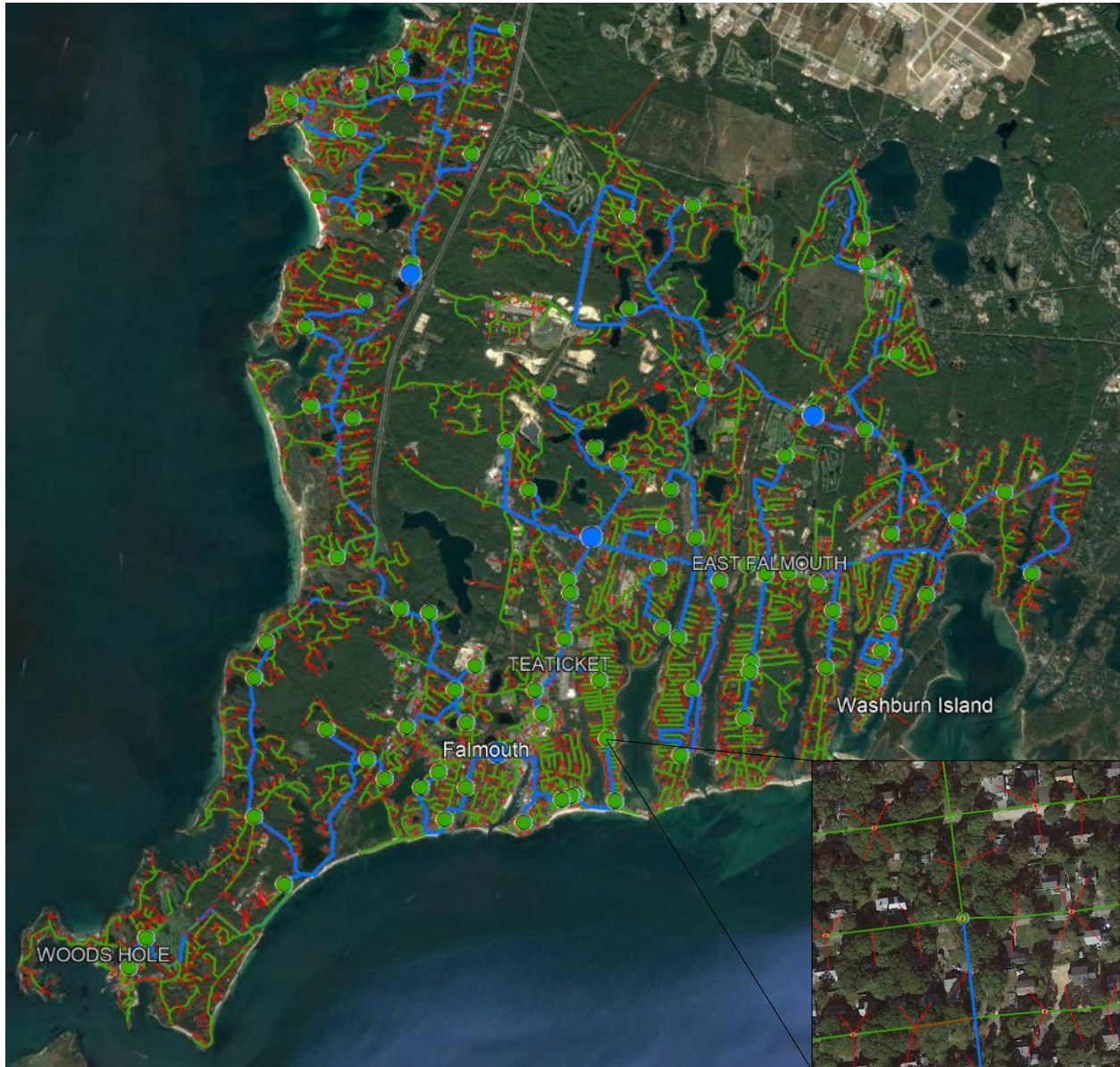
Figure 6: Feeder, Distribution, and Drop Fiber and Hubs
